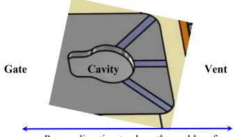
Proper direction to clean the mold surface
